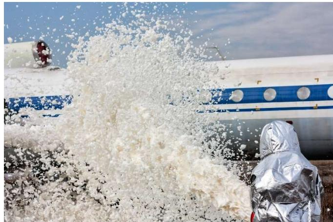
It will generate foam through air aspirating devices to produce a foam expansion rate of between 6 : 1 and 12 : 1 depending upon the equipment.
